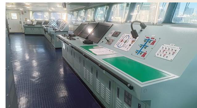
御風輪特別規劃兩座實習駕駛室，並刻意拓寬走道與操作空間，確保學生在觀摩學習時能擁有充裕的視野與動線。Notably, the WIND RIDER features two dedicated training bridges with intentionally widened aisles and operating areas, ensuring students have ample visibility and space to move during observation and hands-on learning.
