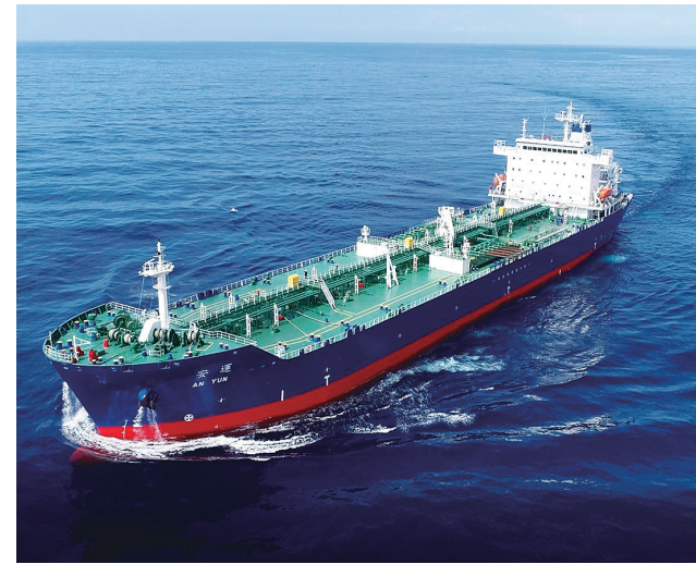
50,000噸級的「安運輸」在設計階段便瞄準2025年第三期船舶能效設計指標（EEDI Phase 3），目標是較基準線降低3成以上的碳排放。The 50,000-ton "Anyun" was designed with a focus on the 2025 EEDI Phase 3 (Energy Efficiency Design Index) standards, aiming to reduce carbon emissions by more than 30% compared to the established baseline.
